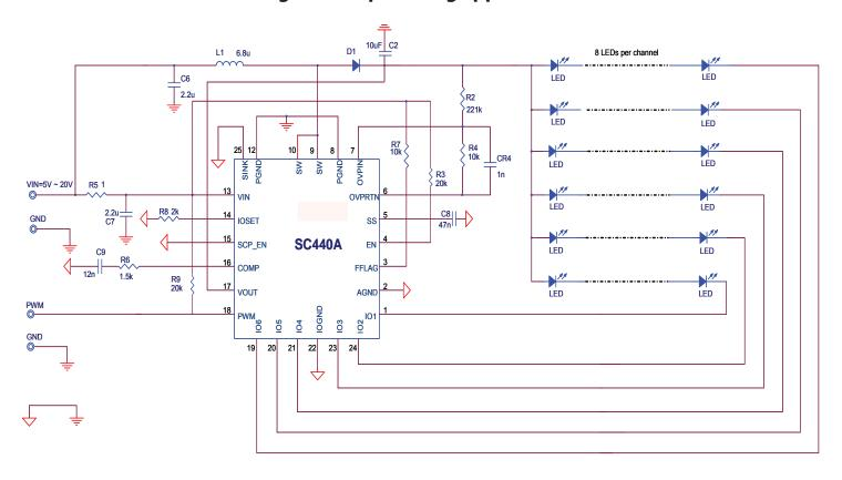
Case 2: Schematic for 5 strings 8 LEDs per string application
