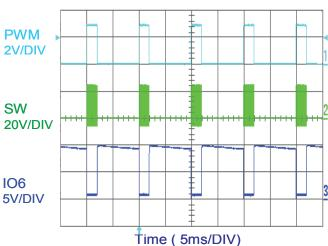
Conditions: VIN = 5V, Load = 30mA x 6 strings, 8 LEDs per string
