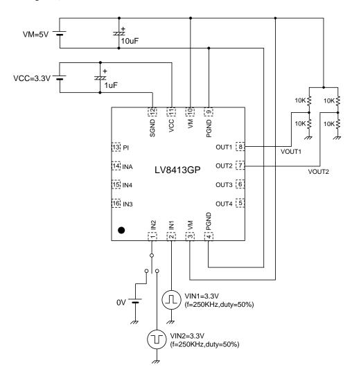
•Macrograph of the PWM switching waveform example \*Please refer to the following Test Circuit diagram2.
