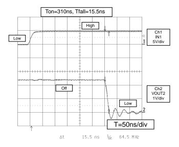
[Fast Decay\_2] VCC=5V,VM=5V,IN2=IN4=0V,IN3=5V VIN1=5V(f=250KHz,duty=50%) OUT1,2=Pull-up&down(10Kohm)
