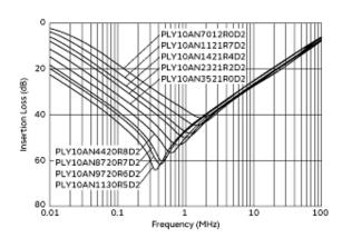
Common Mode Insertion Loss (Typ.)
