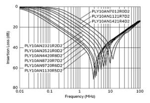
Differential Mode Insertion Loss (Typ.)
