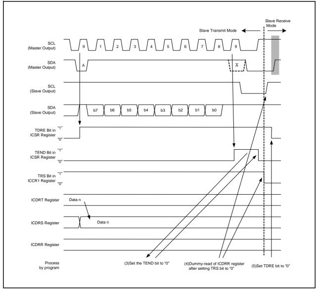
Figure 15.15 Operating Timing in Slave Transmit Mode (I<sup>2</sup>C bus Interface Mode) (2)
