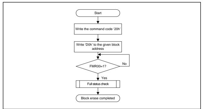
Figure 18.12 Block Erase Command (When Not Using Erase-Suspend Function)
