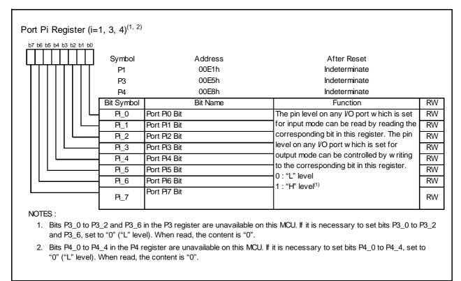
Figure 17.6 P1, P3 and P4 Registers
