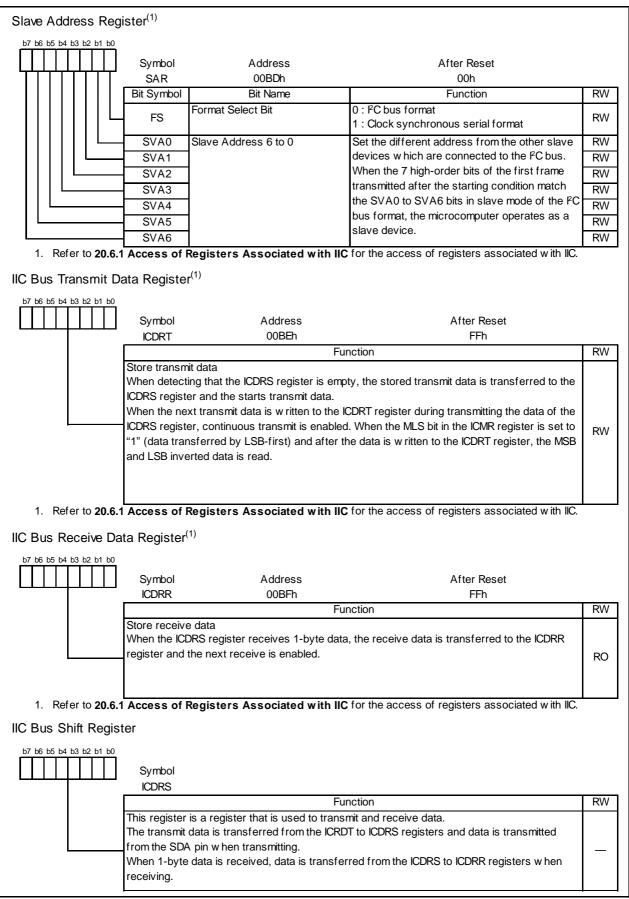
Figure 15.8 SAR, ICDRT, ICDRR and ICDRS Register
