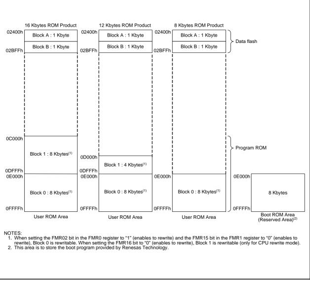
Figure 18.2 Flash Memory Block Diagram for R8C/17 Group
