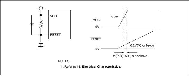
Figure 5.4 Example of Hardware Reset Circuit and Operation
