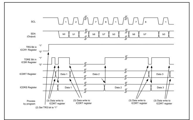
Figure 15.19 Operating Timing in Transmit Mode (Clock Synchronous Serial Mode)
