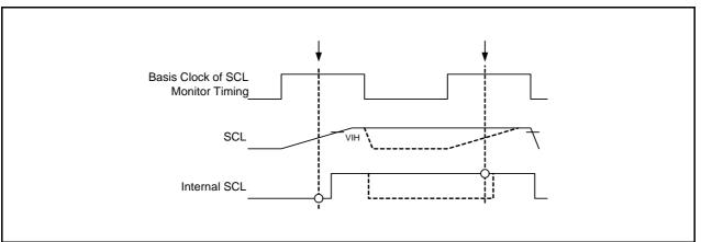
Figure 15.22 Timing of Bit Synchronous Circuit
