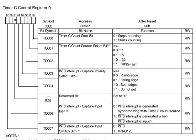
1. Change this bit when the TCC00 bit is set to "0" (count stop).
