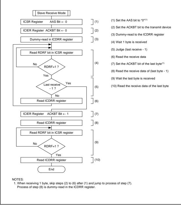
Figure 15.26 Example of Register Setting in Slave Receive Mode
