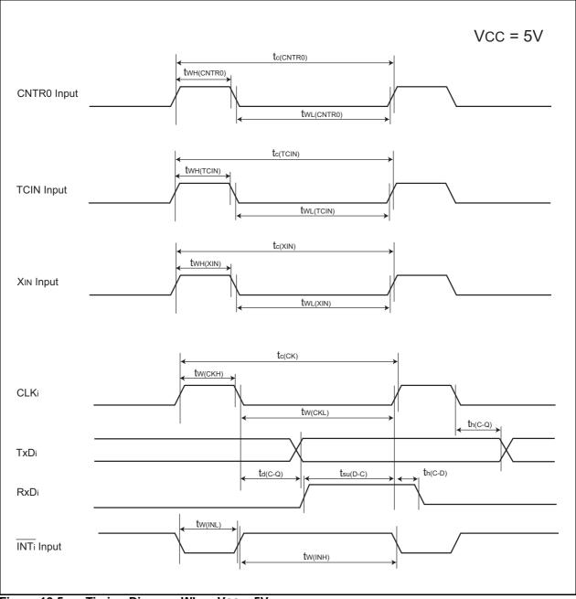
Figure 19.5 Timing Diagram When Vcc = 5V
