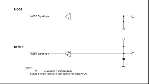
Figure 17.4 Configuration of I/O Pins
