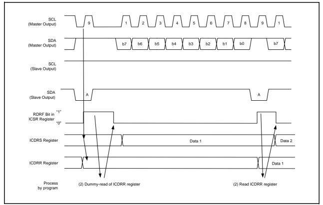
Figure 15.16 Operating Timing in Slave Receive Mode (I<sup>2</sup>C bus Interface Mode) (1)
