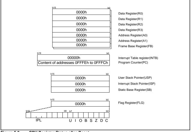
Figure 5.2 CPU Register Status after Reset
