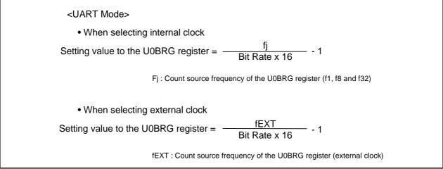
Figure 14.11 Calculating Formula of U0BRG Register Setting Value
