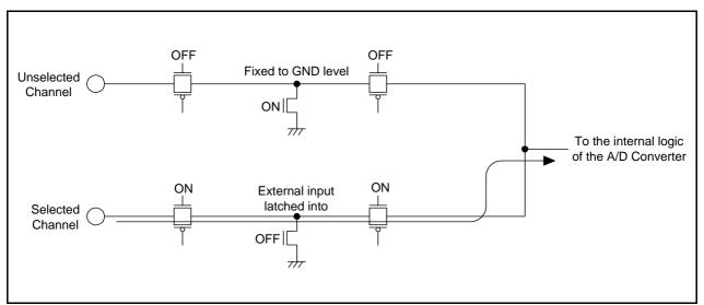
Figure 16.9 Configuration of the Inflow Current Bypass Circuit
