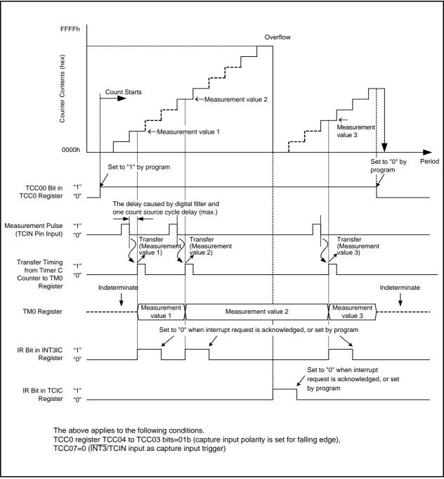
Figure 13.30 Operating Example in Input Capture Mode
