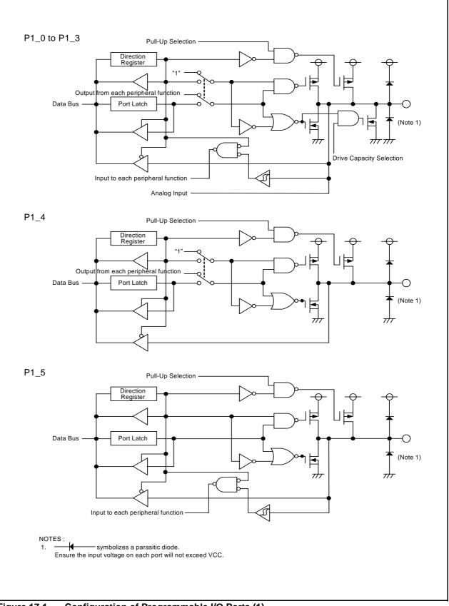
Figure 17.1 Configuration of Programmable I/O Ports (1)
