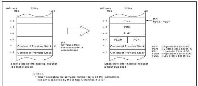
Figure 11.7 Stack State Before and After Acknowledgement of Interrupt Request
