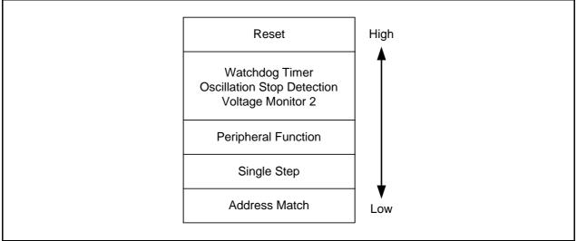
Figure 11.9 Interrupt Priority Levels of Hardware Interrupt
