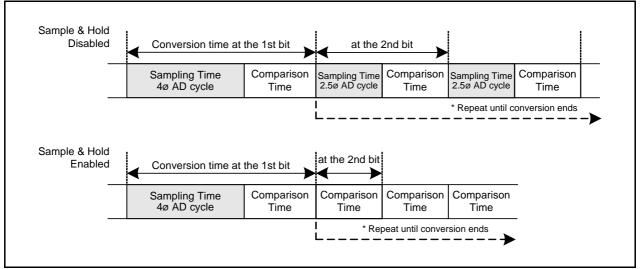
Figure 16.6 Timing Diagram of A/D Conversion
