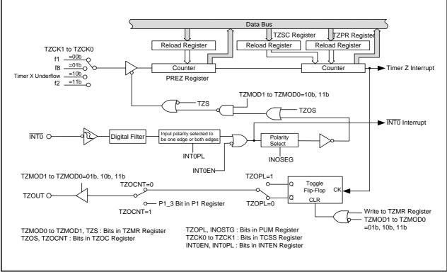
Figure 13.11 Block Diagram of Timer Z
