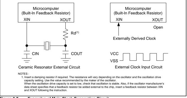
Figure 9.7 Examples of Main Clock Connection Circuit
