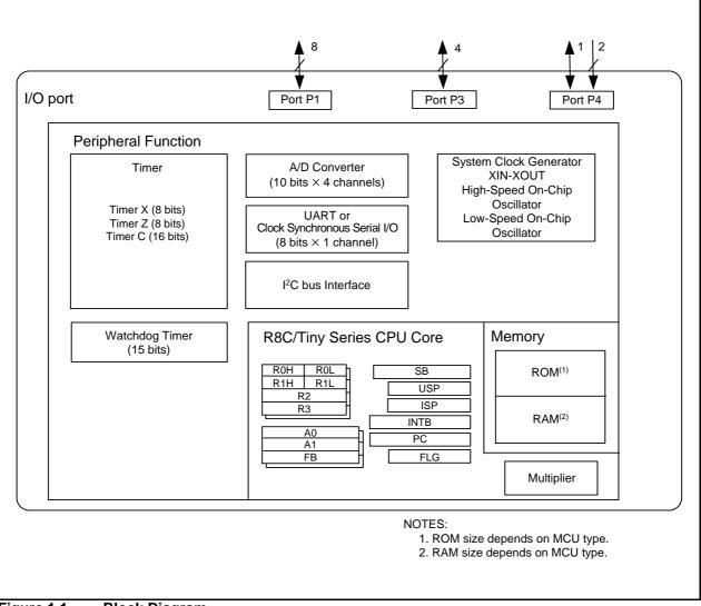
Figure 1.1 Block Diagram
