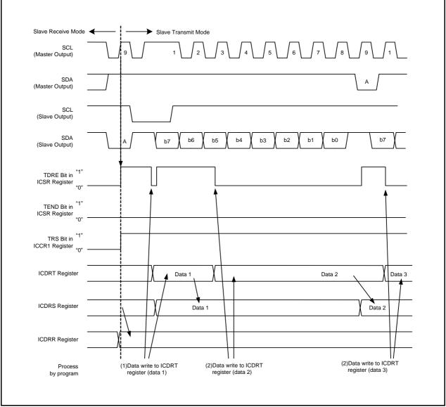
Figure 15.14 Operating Timing in Slave Transmit Mode (I<sup>2</sup>C bus Interface Mode) (1)
