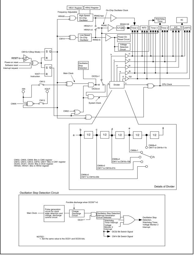
Figure 9.1 Clock Generation Circuit
