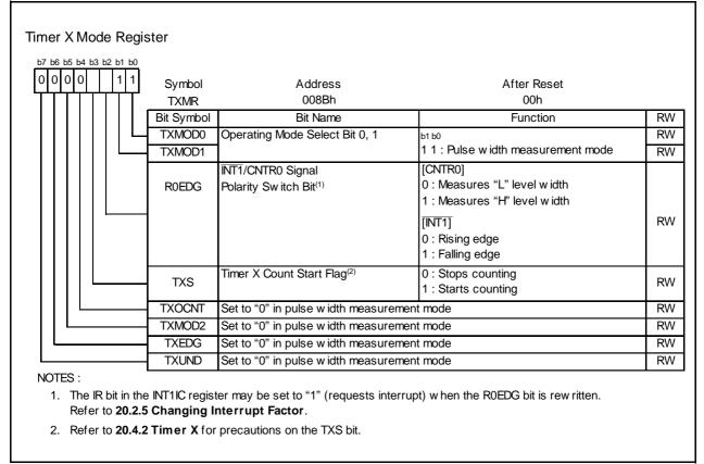
Figure 13.7 TXMR Register in Pulse Width Measurement Mode
