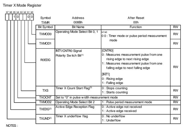
1. The IR bit in the INT1IC register may be set to "1" (requests interrupt) when the R0EDG bit is rew ritten. Refer to 20.2.5 Changing Interrupt Factor.
