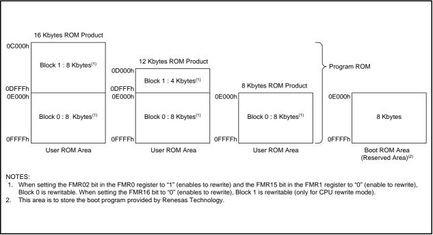
Figure 18.1 Flash Memory Block Diagram for R8C/16 Group
