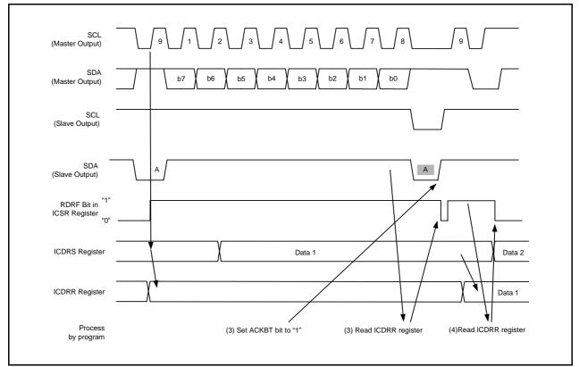
Figure 15.17 Operating Timing in Slave Receive Mode (I<sup>2</sup>C bus Interface Mode) (2)
