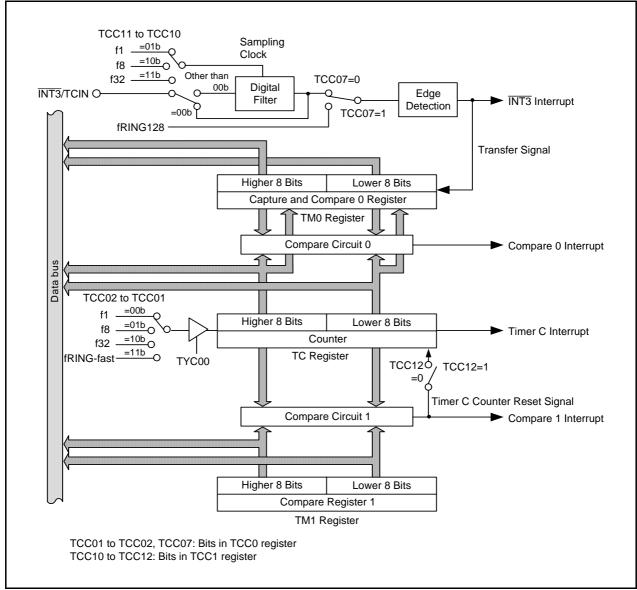
Figure 13.23 Block Diagram of Timer C
