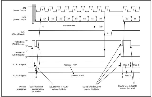
Figure 15.10 Operating Timing in Master Transmit Mode (I<sup>2</sup>C bus Interface Mode) (1)
