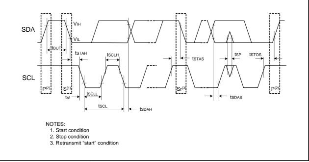
Figure 19.4 I/O Timing of I<sup>2</sup>C bus Interface (IIC)
