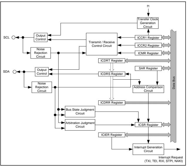
Figure 15.1 Block Diagram of IIC
