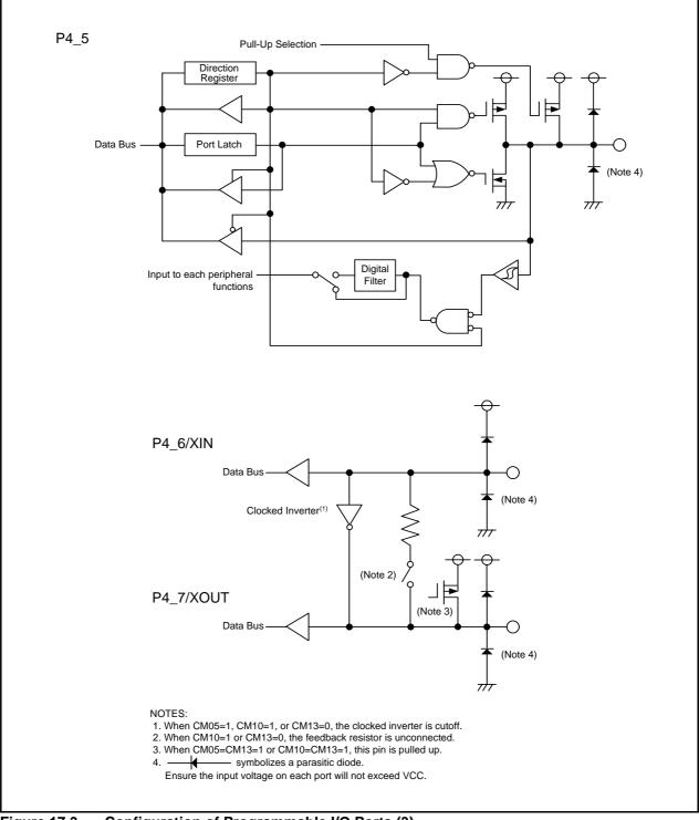
Figure 17.3 Configuration of Programmable I/O Ports (3)
