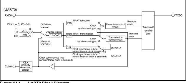
Figure 14.1 UART0 Block Diagram
