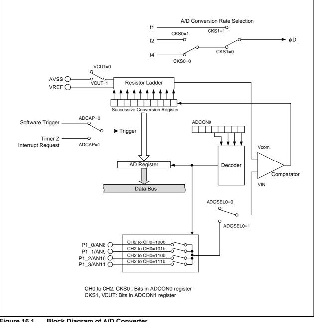
Figure 16.1 **Block Diagram of A/D Converter**
