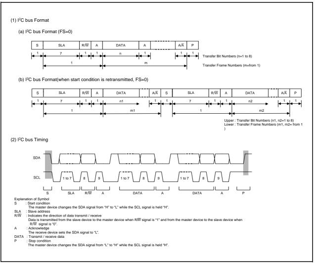
Figure 15.9 I<sup>2</sup>C bus Format and Bus Timing
