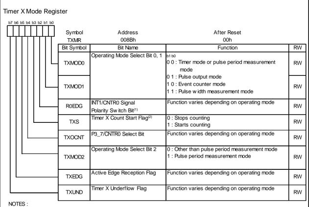
1. The IR bit in the INT1IC register may be set to "1" (requests interrupt) when the R0EDG bit is rew ritten. Refer to **20.2.5 Changing Interrupt Factor.**
