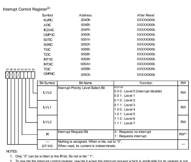
2. To rew rite the interrupt control register, rew rite it when the interrupt request which is applicable for its register is not generated. Refer to **20.2.6 Changing Interrupt Control Registers.**
