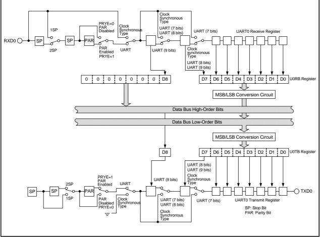
Figure 14.2 UART0 Transmit/Receive Unit
