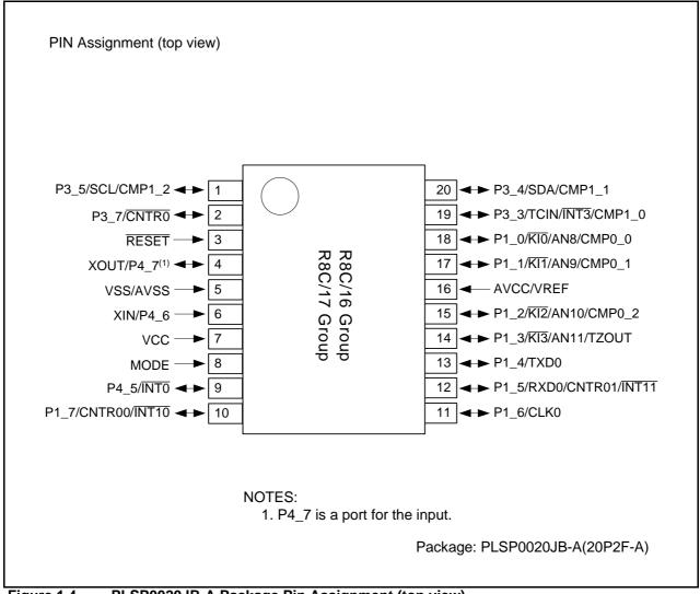
Figure 1.4 PLSP0020JB-A Package Pin Assignment (top view)
