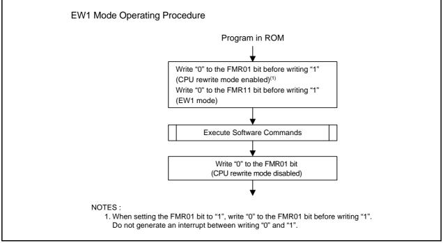
Figure 18.9 How to Set and Exit EW1 Mode
