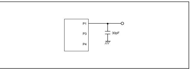
Port P1, P3 and P4 Measurement Circuit Figure 19.1
