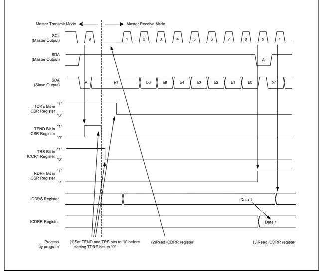
Figure 15.12 Operating Timing in Master Receive Mode (I<sup>2</sup>C bus Interface Mode) (1)
