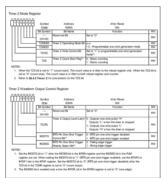
Figure 13.19 TZMR and PUM Registers in Programmable One-Shot Generation Mode
