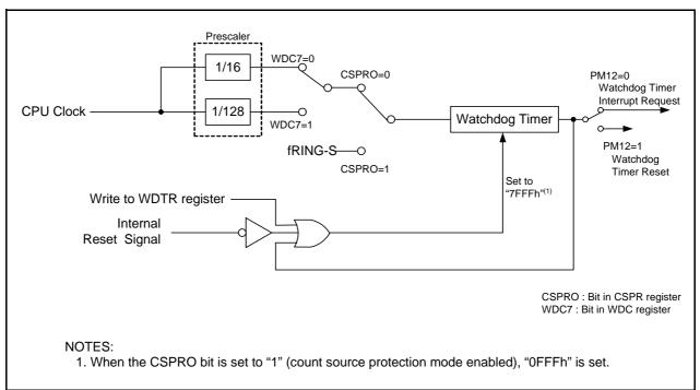
Figure 12.1 Block Diagram of Watchdog Timer
