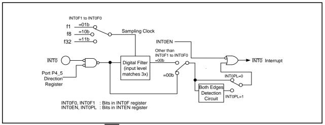
Figure 11.12 Configuration of INT0 Input Filter
