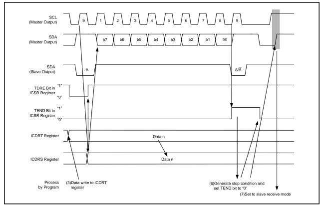
Figure 15.11 Operating Timing in Master Transmit Mode (I<sup>2</sup>C bus Interface Mode) (2)
