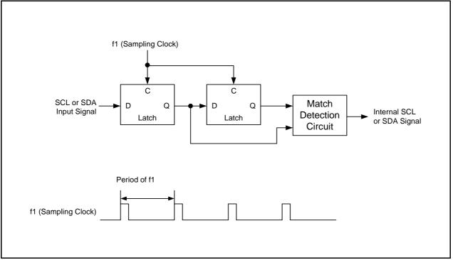
Figure 15.21 Block Diagram of Noise Rejection Circuit
