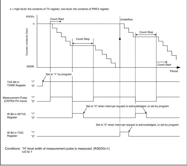
Figure 13.8 Operating Example in Pulse Width Measurement Mode
