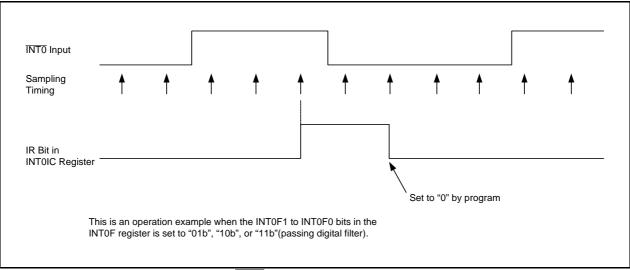
Figure 11.13 Operating Example of INT0 Input Filter
