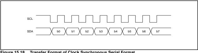
Figure 15.18 Transfer Format of Clock Synchronous Serial Format
