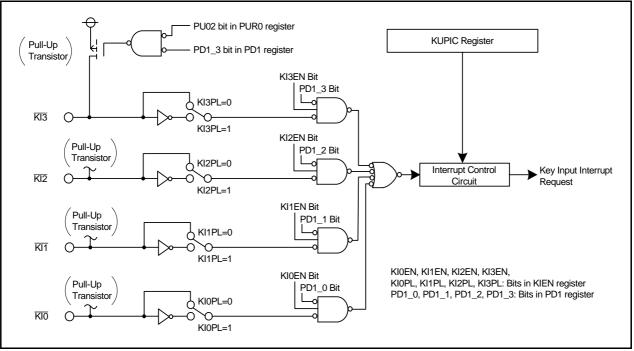
Figure 11.17 Block Diagram of Key Input Interrupt
