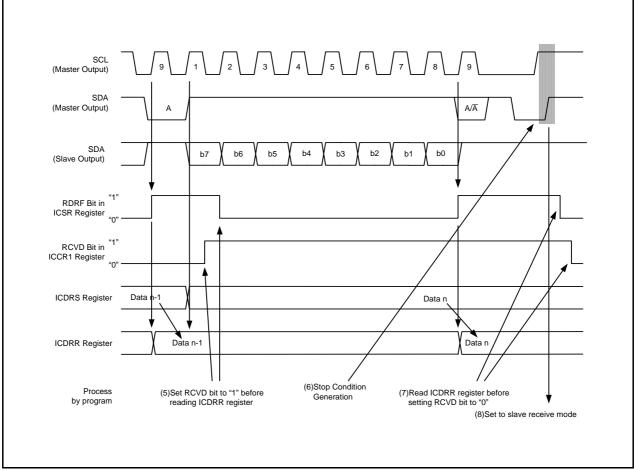
Figure 15.13 Operating Timing in Master Receive Mode (I<sup>2</sup>C bus Interface Mode) (2)
