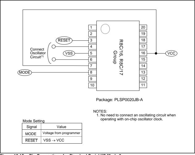
Figure 18.15 Pin Connections for Standard Serial I/O Mode 3
