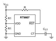
Figure 2. Voltage Divider
