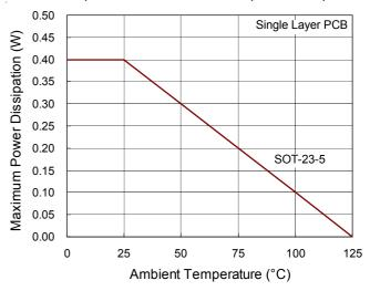
Figure 5. Derating Curve for RT9807 Package
