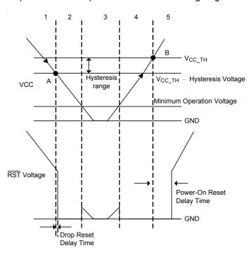
Figure 3. Operation Diagram
