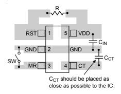
Figure 6. PCB Layout Guide
